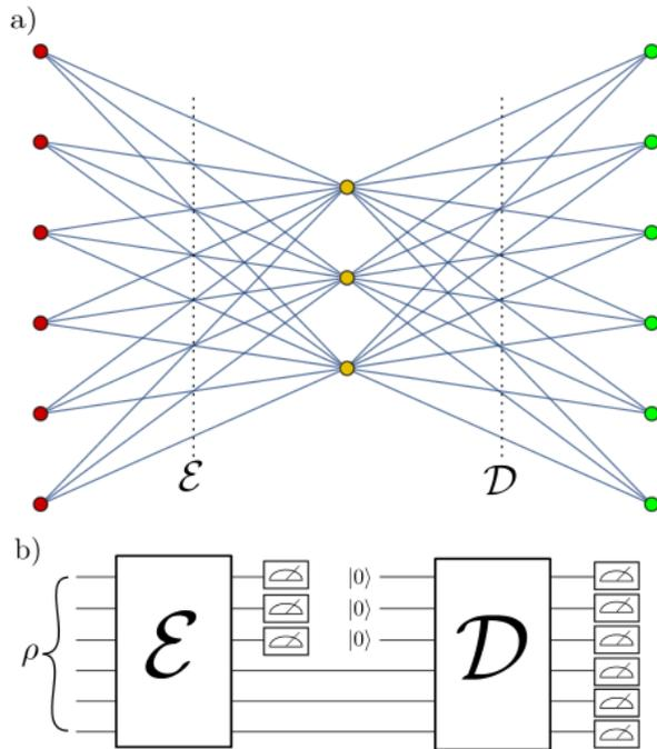
Figure 1. a) A graphical representation of a 6-bit autoencoder with a 3-bit latent space. The map  $\mathcal{E}$  encodes a 6-bit input (red dots) into a 3-bit intermediate state (yellow dots), after which the decoder  $\mathcal{D}$  attempts to reconstruct the input bits at the output (green dots). b) Circuit implementation of a 6-3-6 quantum autoencoder.
