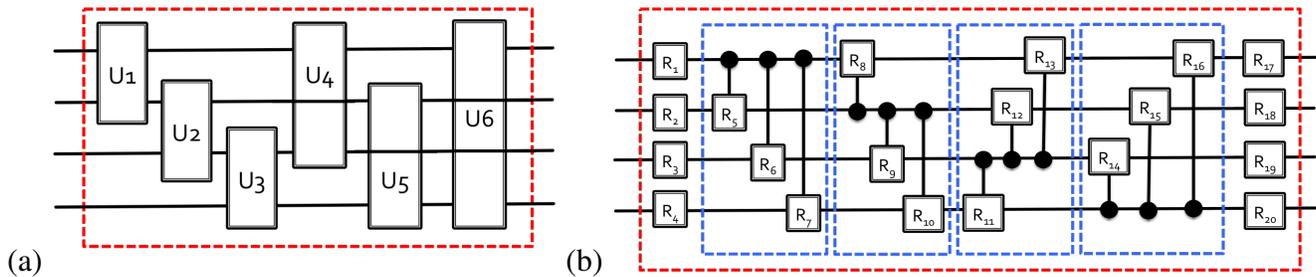
Figure 3. Two programmable circuits employed as autoencoder models: a) Circuit A: a network of all the possible two-qubit gates (denoted by  $U_i$ ) among the qubits. b) Circuit B: a network comprising all the possible controlled general single-qubit rotations (denoted by  $R_i$ ) in a qubit set, plus single qubit rotations at the beginning and at the end of the unit-cell. All the circuits are depicted in the case of a four-qubit input. The unit-cell is delimited by the red dotted line.
